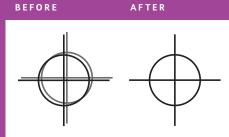
**Auto Alignment Adjustment:** Front-side to back-side image-on-paper registration.
