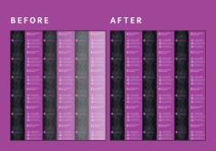
Auto Density Uniformity Adjustment: Lead-to-trail edge and inboard-to-outboard density uniformity.
